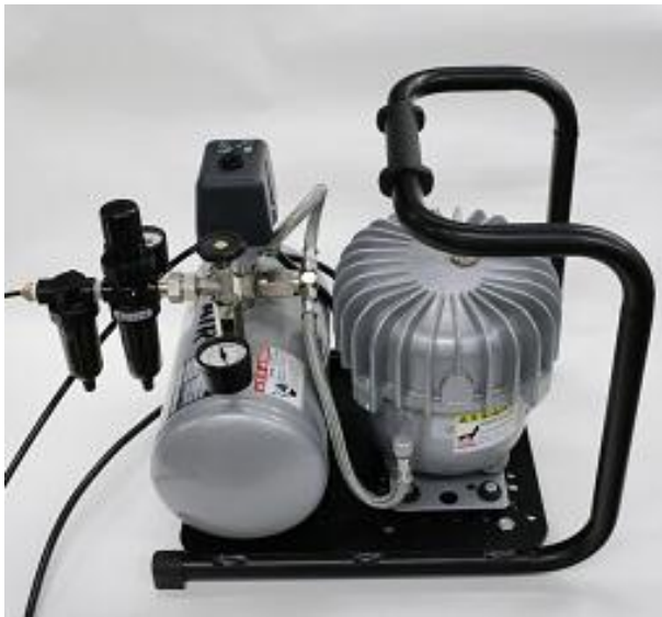
Air compressor (with BMF integrator/mist filter and 2 nd air pressure regulator attached)
