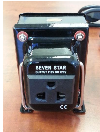
Transformer For air compressor
